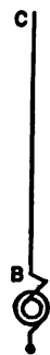
FIG. 2.—Without the lower wire the capacity of the condenser is so small that the alternator could not force an appreciable current to flow in the upper wire.
